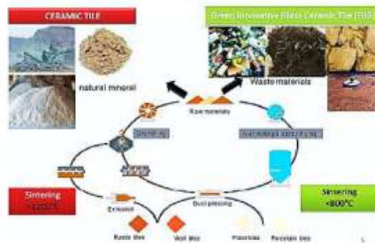
Figure 5: Processing route of a common ceramic tile versus green innovative glass ceramic (GIG) tile
